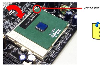
**Note:** If you do not match the CPU socket Pin 1 and CPU cut edge well, it may damage the CPU.
