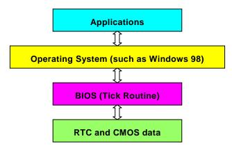
There is a Tick Routine (that goes live around every 50m sec) in the BIOS to keep record of date/time information. In general the BIOS, this Tick Routine does not update the CMOS every time because the CMOS is a very slow device that degrades system performance. The Tick Routine of the AOpen BIOS has 4 digits for year coding, as long as applications and the operating system
