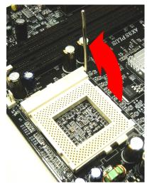
2. Locate Pin 1 in the socket and look for a black dot or cut edge on the CPU upper interface. Match Pin 1 and cut edge, then insert the CPU into the socket.
