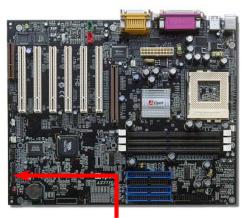
Attach the power LED, EMPI, speaker, power and reset switch connectors to the corresponding pins. If you enable "Suspend Mode" item in BIOS Setup, the ACPI & Power LED will keep flashing while the system is in suspend mode.
