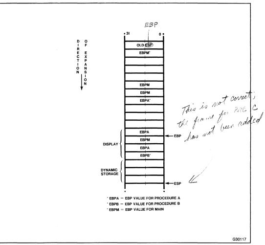
Figure 3-21. Stack Frame for Procedure C at Level 3 Called from B
