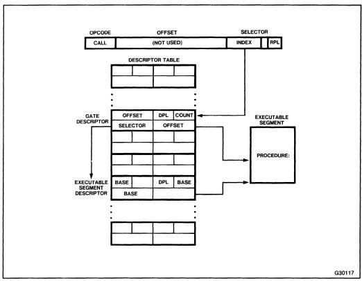
Figure 6-6. Indirect Transfer via Call Gate
