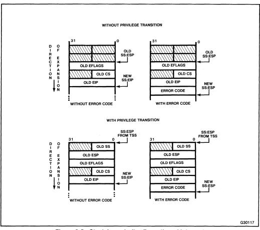
Figure 9-5. Stack Layout after Exception of Interrupt
