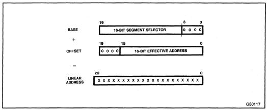
Figure 14-1. Real-Address Mode Address Formation
