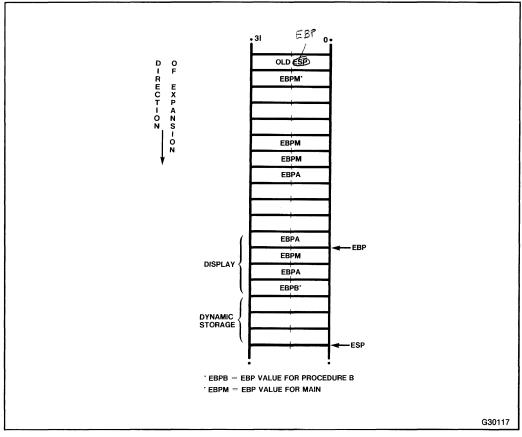
Figure 3-20. Stack Frame for Procedure B at Level 3 Called from A
