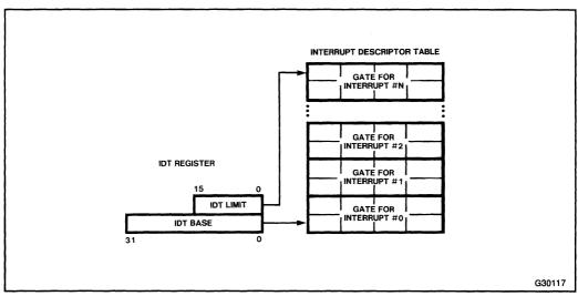
Figure 9-1. IDT Register and Table
