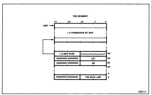
Figure 8-2. I/O Address Bit Map
