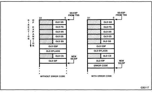
Figure 15-3. PL 0 Stack after Interrupt in V86 Task
