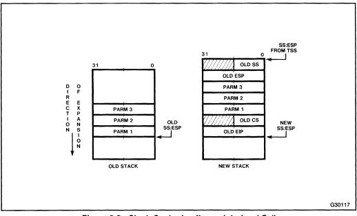
Figure 6-9. Stack Contents after an Interlevel Call
