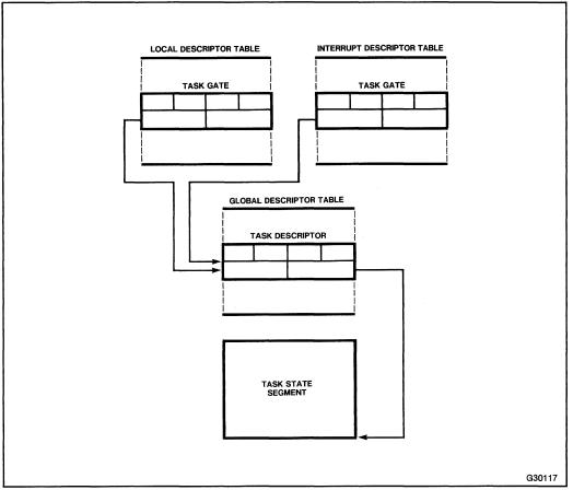
Figure 7-5. Task Gate Indirectly Identifies Task
