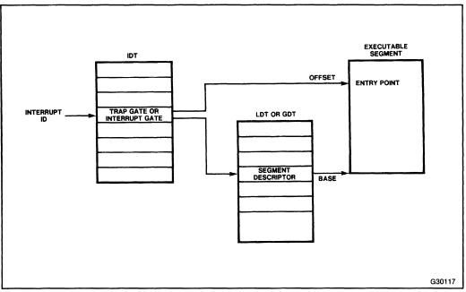
Figure 9-4. Interrupt Vectoring for Procedures
