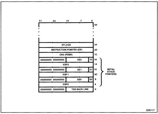
Figure 6-8. Initial Stack Pointers of TSS
