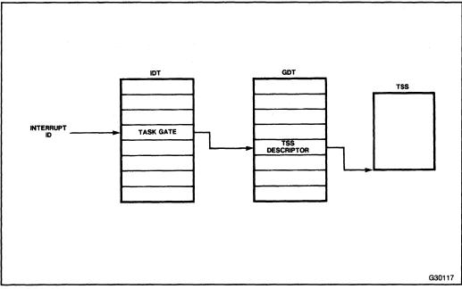
Figure 9-6. Interrupt Vectoring for Tasks
