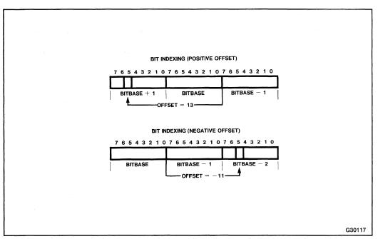
Figure 17-4. Memory Bit Indexing
