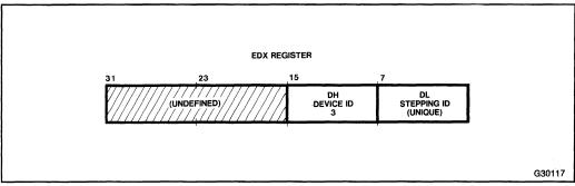
Figure 10-1. Contents of EDX after RESET
