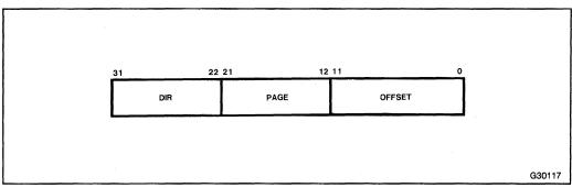
Figure 5-8. Format of a Linear Address
