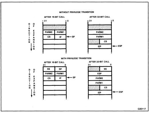
Figure 16-1. Stack after Far 16-Bit and 32-Bit Calls
