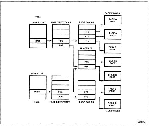
Figure 7-6. Partially-Overlapping Linear Spaces
