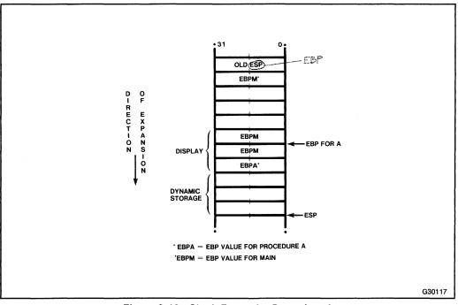
Figure 3-19. Stack Frame for Procedure A
