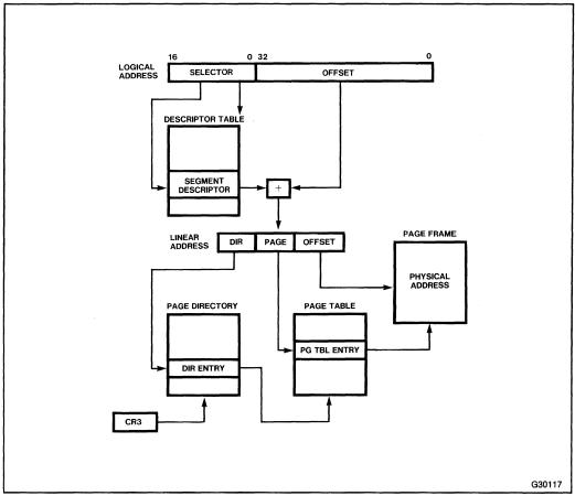
Figure 5-12. 80386 Addressing Mechanism
