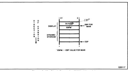
Figure 3-18. Stack Frame for MAIN at Level 1
