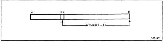
Figure 17-3. Bit Offset for BIT[EAX, 21]
