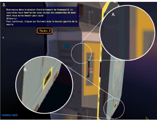
Figure 18: Real World Example of 4 sub-sample RGSS (a) shows a near vertical edge. (b) shows a near 45° edge.
