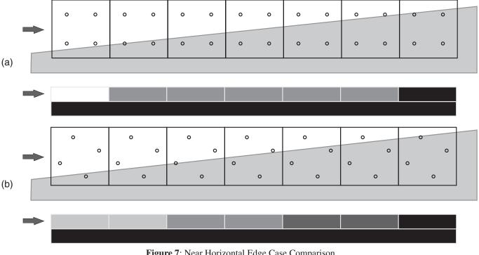
Figure 7: Near Horizontal Edge Case Comparison (a) OGSS (b) RGSS
