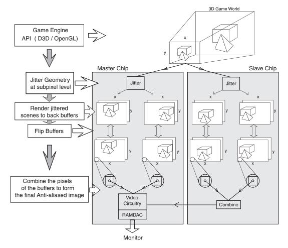
Figure 6: Overview of the Rotated Grid Super-sampling Method.
