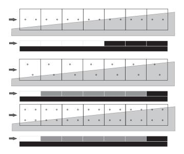
**Figure 14**: Quality of 2 Sub-sample Super-sampling From top to bottom we have 2 Sub-sample OGSS, 2 Subsample RGSS and 4 Sub-sample OGSS.
