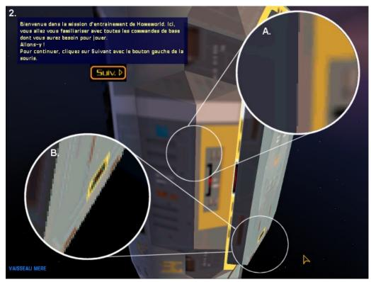
Figure 17: Real World Example of 2 sub-sample RGSS (a) shows a shows a near vertical edge. (b) shows a near 45° edge.
