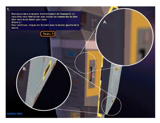
Figure 16: Real World Example of 4 sub-sample OGSS(a) shows a Bad Case Angle resulting in poor quality(b) shows a normal Edge Angle resulting in acceptable quality
