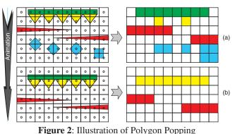
(a) Finely detailed representation on the left, sampled version with missing polygons and details on the right.
