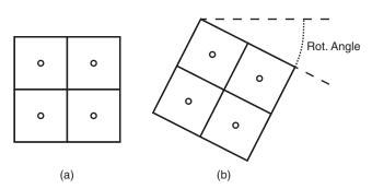
Figure 3: Illustration of different sampling grids (a) Ordered Grid as used by the OGSS method. (b) Rotated Grid as used by RGSS method.
