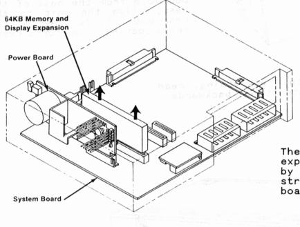
The 64K memory and display expansion board can be removed by gently pulling the board straight up from its system board connector.
