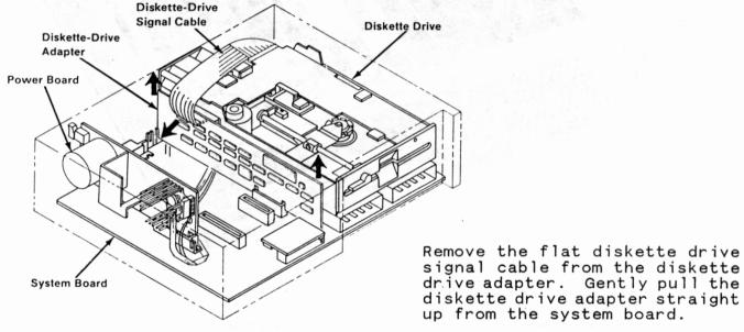
Remove the diskette drive power cable and the flat diskette drive signal cables from the rear of the diskette drive. Note that the power cable can be installed only one way. Also note that the signal cable is keyed making it impossible to install incorrectly.
