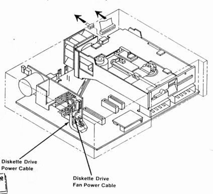
Gently disconnect the diskette drive power cable and diskette drive fan power cable from the internal power supply board. Gently pull the power board straight up from its system board connector.
