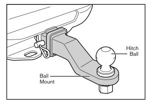
balls are available in a number of weight capacities and sizes. Most hitch balls have the size stamped on the top of the ball. The required hitch ball size is stamped on most trailer
