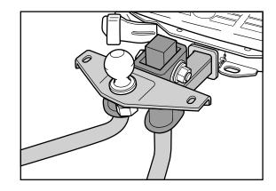
recommended if you plan to tow trailers with a maximum weight over 5,000 lbs. This ball mount includes a 2<sup>5</sup>/16" hitch ball rated for up to 10,000 lbs., and is available through your NISSAN dealer.
